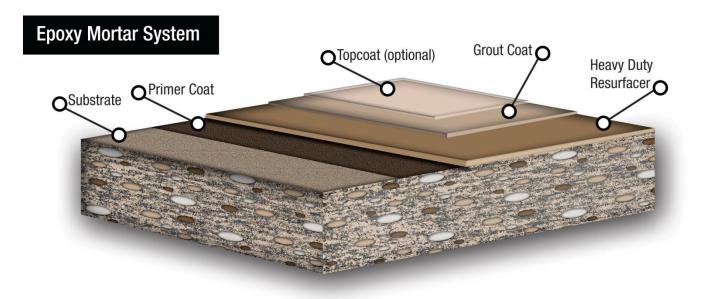
RS-41CR is a Heavy-Duty Acid/Chemical Resistant Epoxy Mortar Flooring System is a troweled, high strength concrete resurfacing material. It is used for environments requiring an industrial grade protective floor or when a concrete floor has sustained damage requiring a 3/16" to 1/4" surface restoration.
